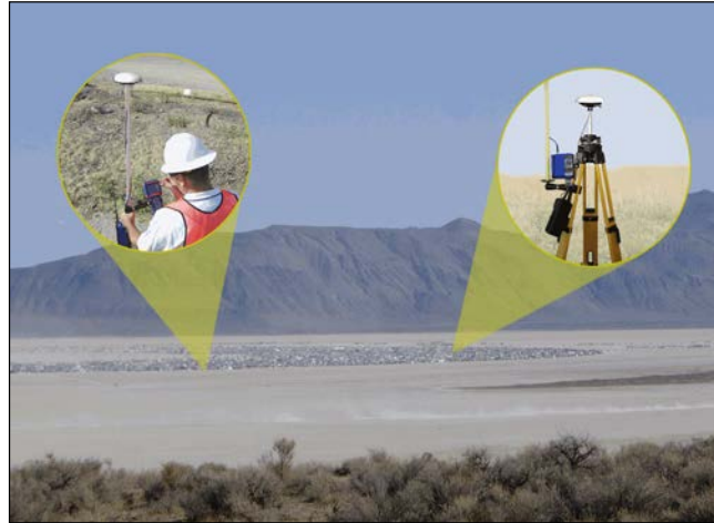
Figure 110: RTK Setup – Good Line of Sight
