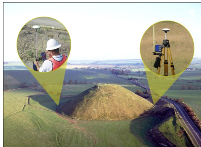
Figure 111: RTK Setup – Poor Line of Sight
