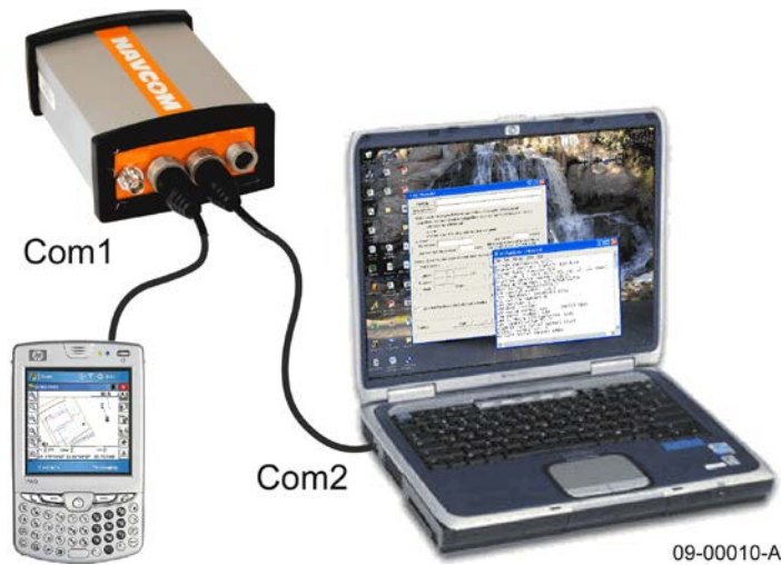
Figure 109: Communication Port Connections
