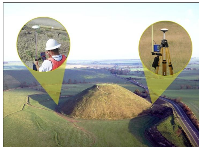
Figure 58: RTK Setup – Poor Line of Sight
