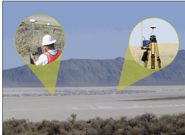
Figure 57: RTK Setup – Good Line of Sight
