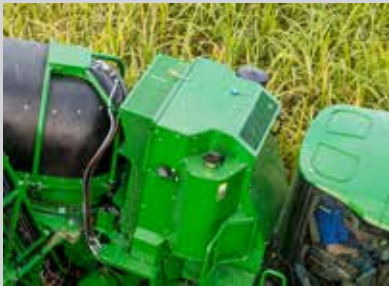
The reversible fan automatically keeps the cooling package clean and with the New variable speed control it will maintain the engine operating at the appropriate temperature to optimize engine performance.
