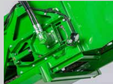
The exclusive grease cylinder facilitates elevator chain tension adjustment.
