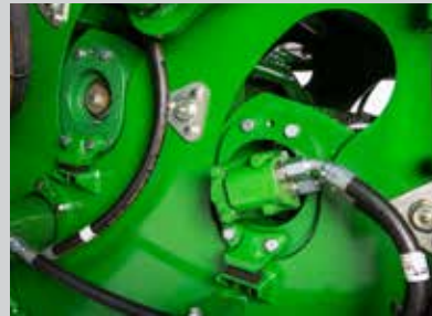
Access is easy with externally mounted bearings and bolt-on cradle stops with rubber shock absorber pads.
