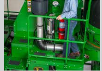
Service platforms have non-skid surfacing and are surrounded by handrails for safe access.
