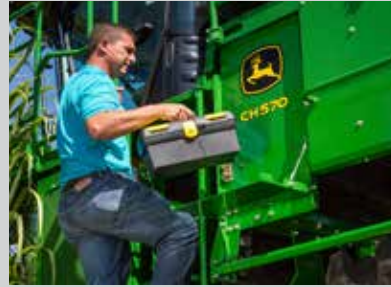
New convenient foldable shelf facilitates access when carrying a tool box or other large miscellaneous item.
