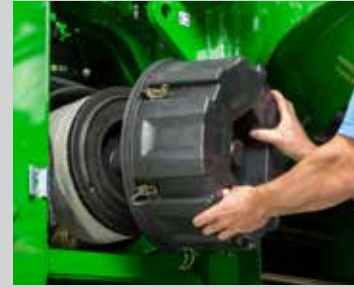
New air filter assembly is better protected and the hood is easier to grip.
