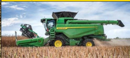
Easily maintain a consistent feed rate with Ground Speed Automation<sup>1</sup>. It's a dynamic ground speed control that's based on your inputs and operator-defined limits on variables such as grain loss, engine power, and drum pressure.
