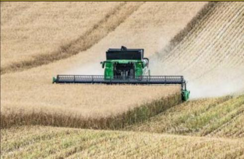
Terrains may vary, but your cleaning shoe performance shouldn't. That's why we gave the T6 800 automated terrain adjustment<sup>1</sup>. Using pitch angle data from the integrated StarFire Receiver, the combine automatically calculates needed changes in the fan speed, chaffer and sieve opening to prevent cleaning shoe over-blow and material being moved too fast — or not at all.
